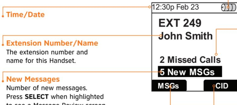
Figure 15. SB67040 Cordless Handset Idle Screen
