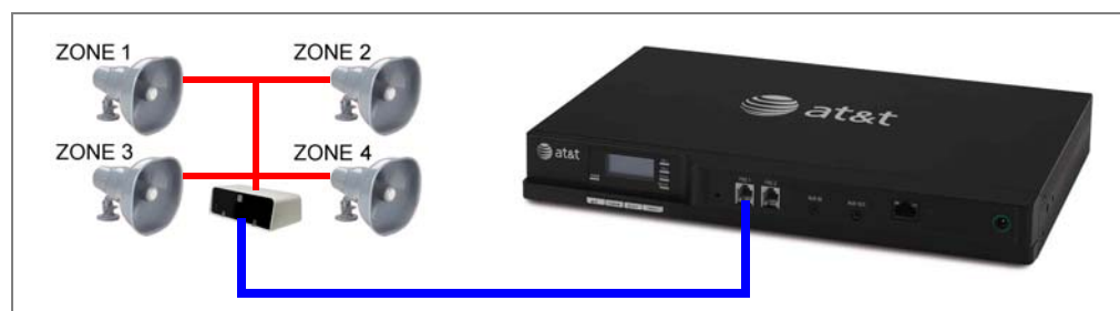
Figure 7. Multiple-Zone Overhead Paging on FXS Port
