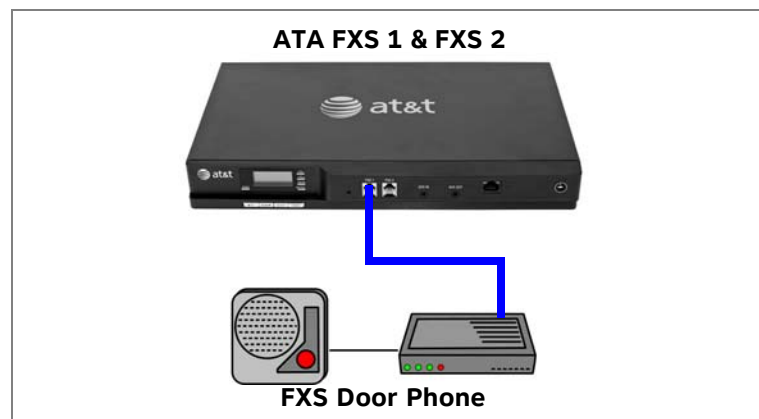
Figure 8. Station Port (FXS) Door Phone Connection
