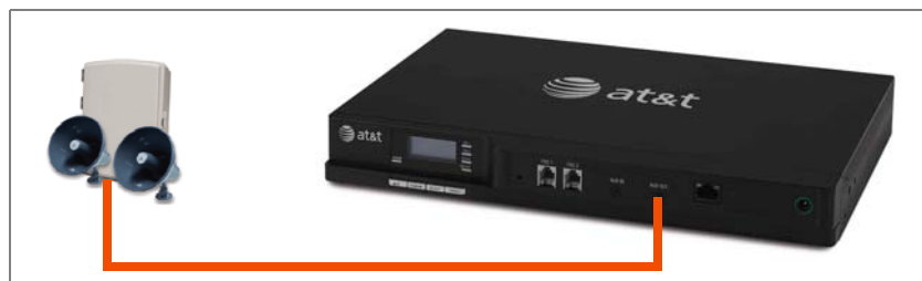
Figure 5. Single-Zone Overhead Paging on AUX OUT Jack
