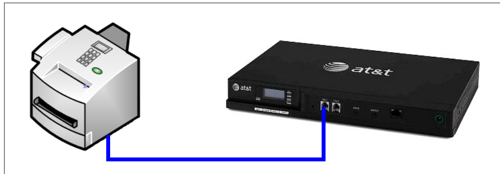
Figure 10. Fax Machine Connected to FXS Port
