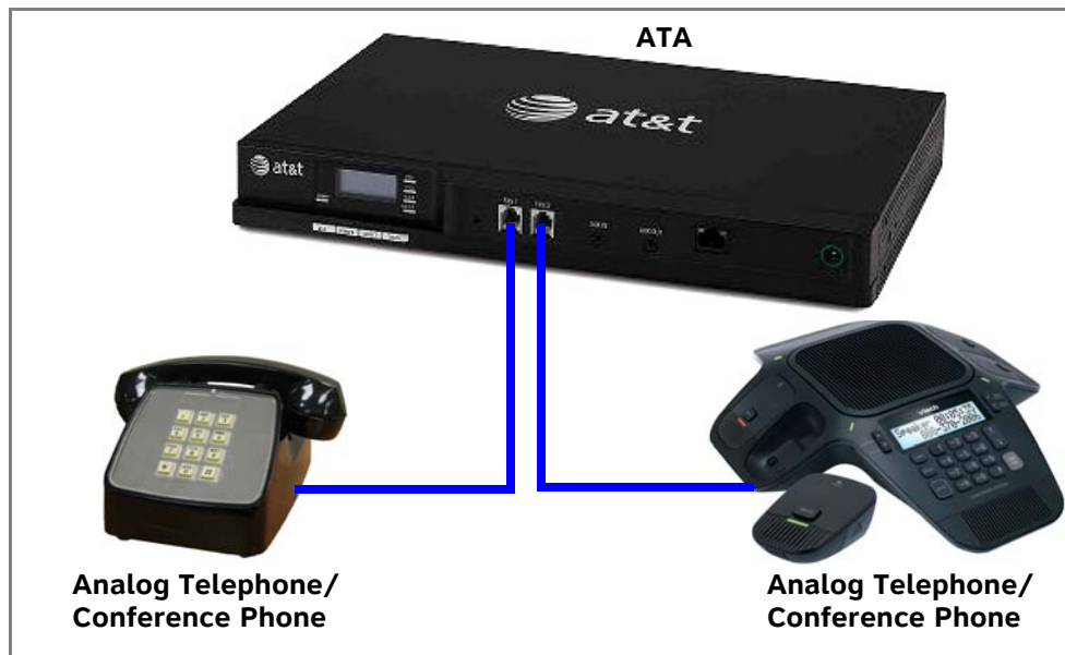
Figure 24. ATA Analog Telephone Connections
