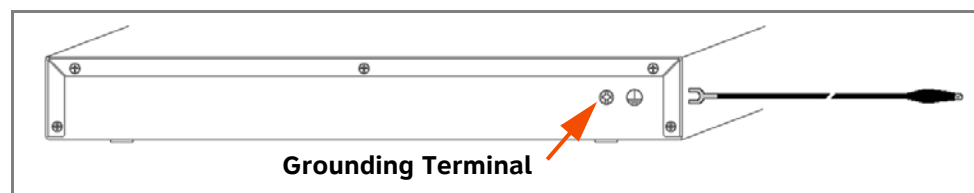
Figure 13. T1 Gateway, SIP Gateway, and ATA Grounding
