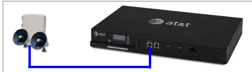
Figure 6. Single-Zone Overhead Paging on FXS Port
