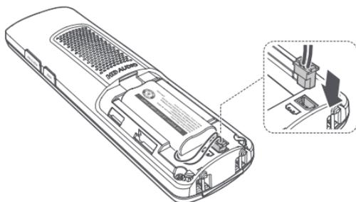
2. Align the cover flat against the battery compartment, then slide it upwards until it clicks into place.
