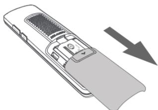
To replace the battery, press the tab and slide the battery compartment cover downwards. Lift out the old battery and disconnect it from the handset. Follow the instructions to install and charge a new battery.
