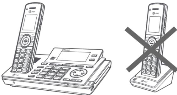
For registration, put the handset on the telephone base, not the handset charger.
