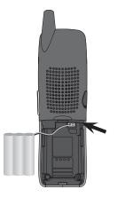
Plug the battery pack connector into handset.
