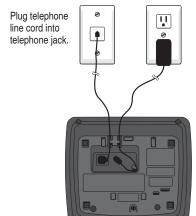
Plug the large power adapter into an electrical outlet not controlled by a wall switch.
