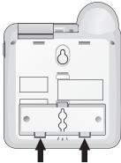
Press the tabs down to remove the bracket
