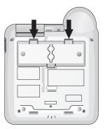
2. Install batteries to provide power for the **AUDIO ASSIST**, **MUTE** and **4***D* lights. Press the battery cover tabs as shown below to open the battery compartment. Install three new alkaline AA batteries (not included). Make sure to follow the polarity guide in the battery compartment. Replace the cover.
