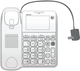
Telephone base with power adapter installed
