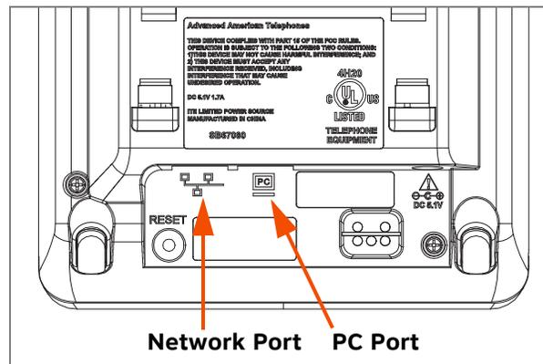
**Figure 4. Expansion Module Network and PC Ports**
