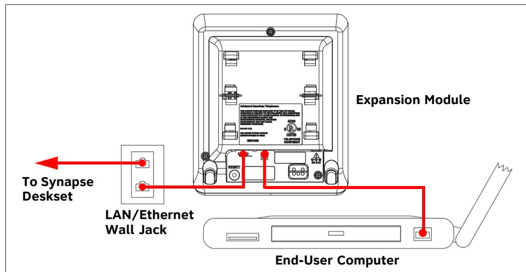
3. Plug another Cat.-5 Ethernet cable into the PC port on the Expansion Module.
