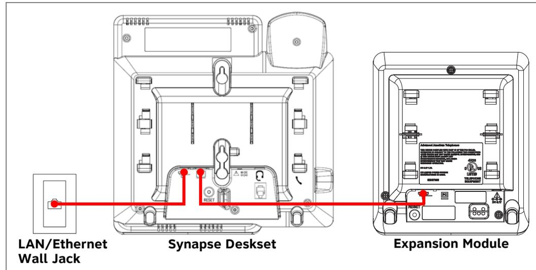
**To connect the Expansion Module without a shared network connection with a Deskset:**
