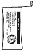
Battery for cordless handset (One for CL81101) (Two for CL81201/CL81211) (Three for CL81301)
